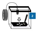
Place **P-surface 141** with the PPprint logo upwards on your printer bed and fix it with gentle pressure using the **P-roller 621**. You have also the option to adhere **P-surface 141** to your printer bed by using **P-adhesive 220**.
