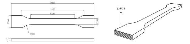
FLEXURAL TESTING SPECIMEN
