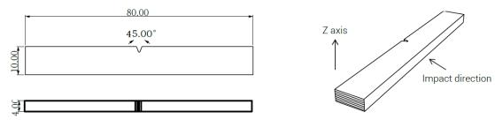
Impact testing specimen; ASTM D256 (ISO 179, GB/T 1043)
