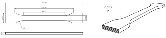
Tensile testing specimen; ASTM D638 (ISO 527, GB/T 1040)
